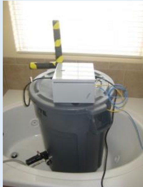
This device, built by EPRI’s Chuck Thomas, simulates human heat and sweat.
