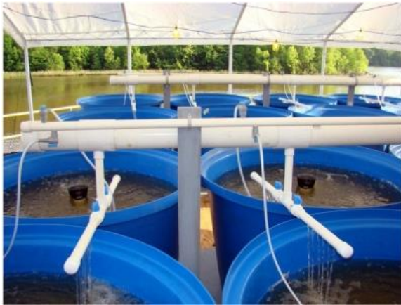
In this aquarium facility at the Barry plant, fish are held for 24 to 48 hours for survival testing.
