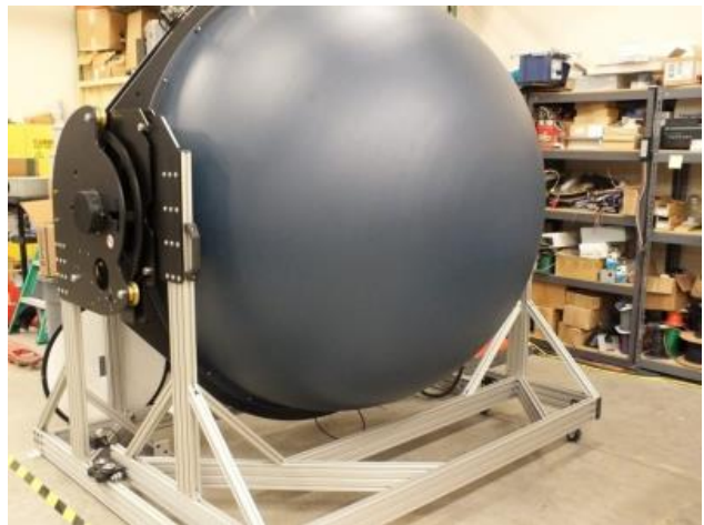
This two-meter integrating sphere in EPRI’s lighting lab is used to evaluate illuminance and other lighting characteristics.
