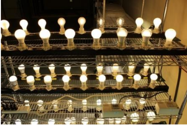
Evaluation of power cycling and lifespan of various screw-in lamps in EPRI's lighting lab.
