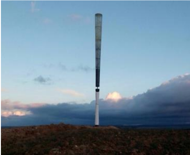
Photo courtesy of Vortex Developed by Vortex, these prototypes of bladeless cylindrical turbines generate electricity by oscillating in the wind.
