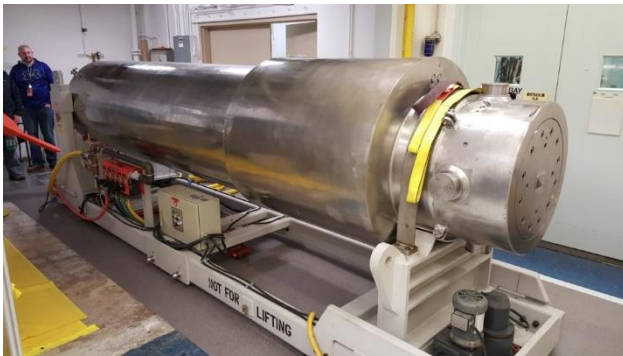
Photo courtesy of Oak Ridge National Laboratory, U.S. Department of Energy The shipping cask with sister fuel rods after it arrived at Oak Ridge National Laboratory in early 2016. Researchers will compare the physical state of the sister rods and the rods inside a specially instrumented dry storage cask after a decade of storage.
