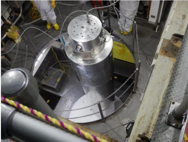
Photo courtesy of Dominion Virginia Power Technicians at Dominion Virginia Power's North Anna nuclear plant prepare a shipping cask containing fuel rods from high burnup assemblies for shipment to Oak Ridge National Laboratory. These "sister rods" are similar to ones that will be loaded inside a specially equipped dry storage cask as part of an EPRI-led 10-year demonstration project.
