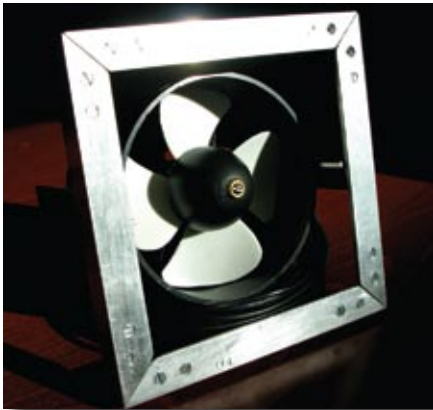
The UNCC team used an off-the-shelf piezoelectric flashlight, a small photovoltaic cell, and a propeller for a hobbyist's remote-controlled airplane to harvest energy from vibration, sunlight, and wind, respectively.
