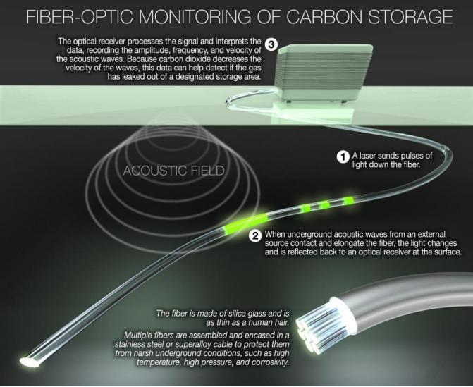
This graphic shows how fiber-optic monitoring of carbon storage works.
