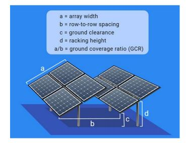
Module choice is also significant. Monofacial modules generate electricity using sunlight incident only on the top side of the panel. Bifacial modules, by contrast, can utilize sunlight received on both sides of the panel. Planting white or light-colored pollinator plants can increase the amount of sunlight reflected off the ground or albedo. Using bifacial modules in conjunction with such high-albedo vegetation can boost the performance of a solar power plant.
